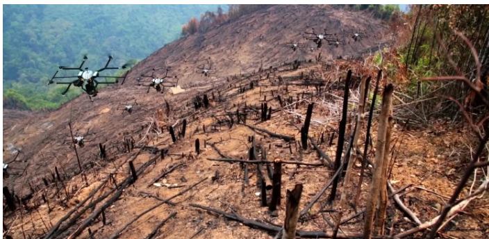
A drone swarm drops seeds on a steep mountainside.
