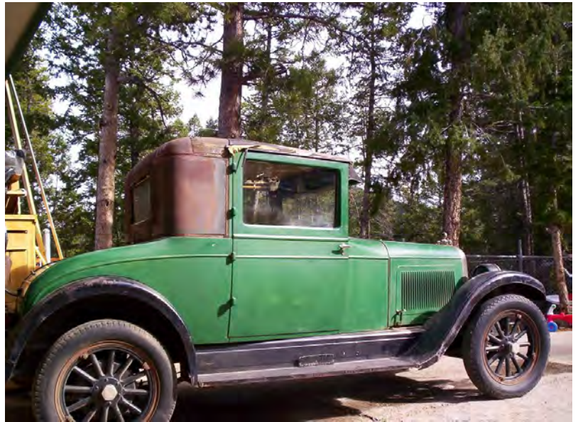
1926 Overland car before restoration. Canvas top missing. Painted with latex house paint.
