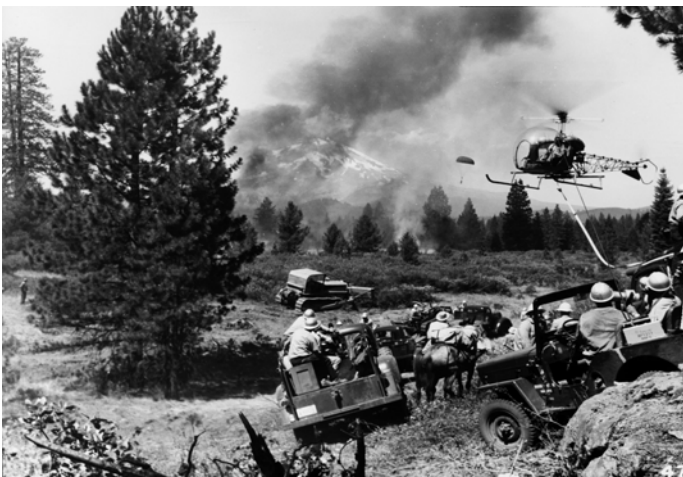
Specially staged photo showing fire equipment used in controlling forest fires – helicopter laying hose, motor equipment and pack horse for getting into back country, bulldozer, and Smokejumper in background. Shasta-Trinity-National Forest, California. 1955 (Forest Service photo by Donald J. Lewis)
