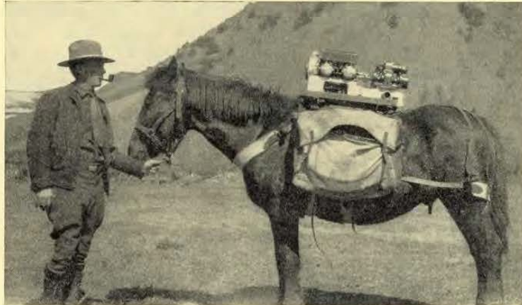
A Pacific Marine Portable Fire Pump mounted on Saddle with Special Steel Frame in place on horse ready for action. Hose is run to creek and to fire from pump, making possible the use of a pressure stream of water on the blaze.
